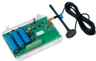
EWK2 - wireless signal repeater
